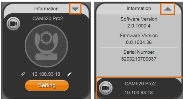
8. **Camera:** Click the camera icon to view the camera live view. IP address is displayed as well. Click the X icon to close the camera live view. If the live video did not appear, please check the camera and the laptop/PC connection to make sure all are correct and well connected. The resolution of this small live view is 640x480 resolutions.
